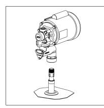
5. To prevent pressure buildup and possible leaks through the ball valve, make sure the tank is vented.
