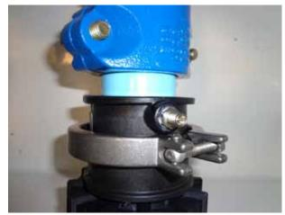
Figure 4: Clamp in Position
