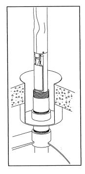
**CAUTION:** No obstruction can be within 13" from the center of the riser pipe or the valve will not operate properly.
