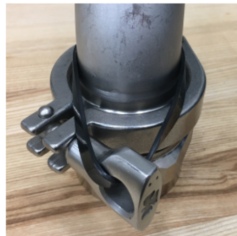
Correct EZ-Fit zip tie installation
